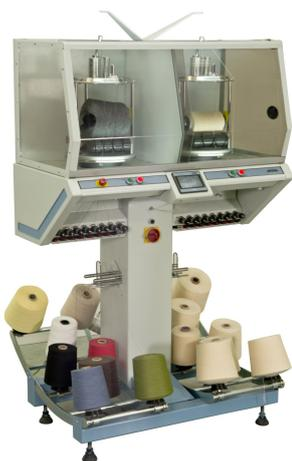
**DirectTwist-2B6** is the basic model with **6 inch take-up cone**. Only the lower plate is turning.
